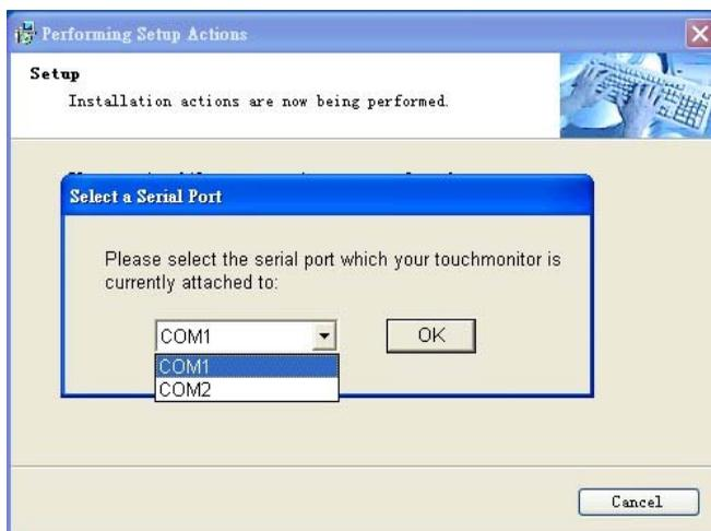
8. Select the serial port and click [Finish] to start the four-point calibration.
